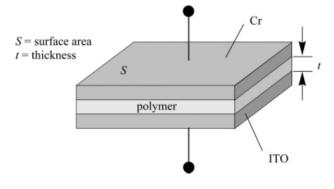
**Figure 8** Schematic representation of sandwich-type capacitor. The cast film was sandwiched between the ITO and Cr electrodes.
