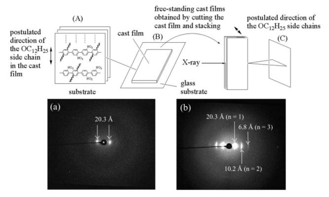
**Figure 7** X-ray diffraction patterns measured for solution-cast film of **P2**: (a) as-prepared film at r.t; (b) after annealing at  $200^{\circ}$ C. The direction of the X-ray beam is shown in the drawing above the diffraction patterns.
