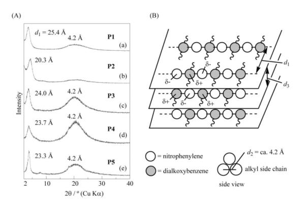
Figure 6 (A) Powder XRD patterns of (a) P1, (b) P2, (c) P3, (d) P4, and (e) P5. (B) Schematic packing structure of the polymer in the solid state.
