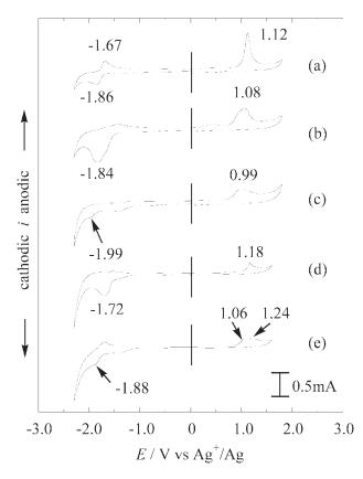
**Figure 4** CV charts of (a) **P1**, (b) **P2**, (c) **P3**, (d) **P4**, and (e) **P5** films on a Pt plate in an acetonitrile solution of  $[Et_4N]BF_4$  (0.10*M*) under N<sub>2</sub>. The sweep rate is 50 mV s<sup>-1</sup>.
